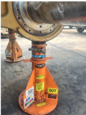
Figure 3 Stands are being used on a concrete pad
